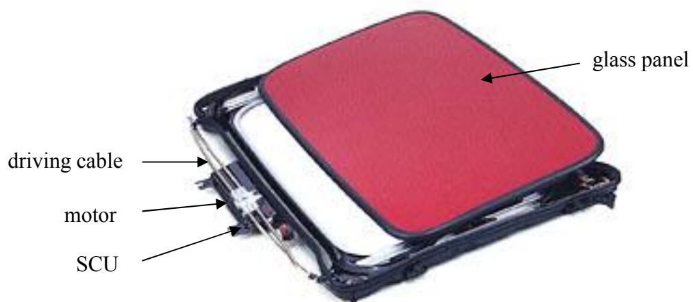
Figure 2-1: A typical sunroof system
