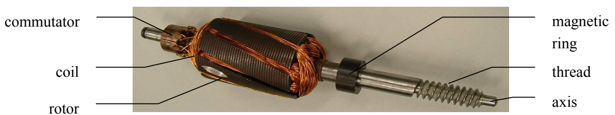
Figure 5-2: A motor rotor
